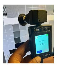
Model SC-830 Designed for Display Surface Luminance Measurement
